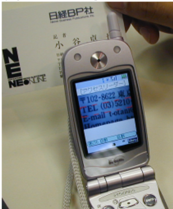
Fig 2 New OCR and Infrared Communication Functions in Mova N504iS (a) Reading character information from a business card with the OCR function. (b) Can also be used as a TV remote controller.
