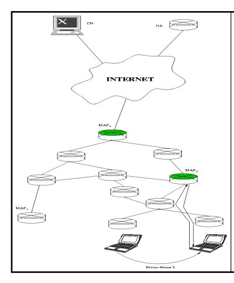
•Then for each movement inside, the binding procedure ends at the cross-over MAP
