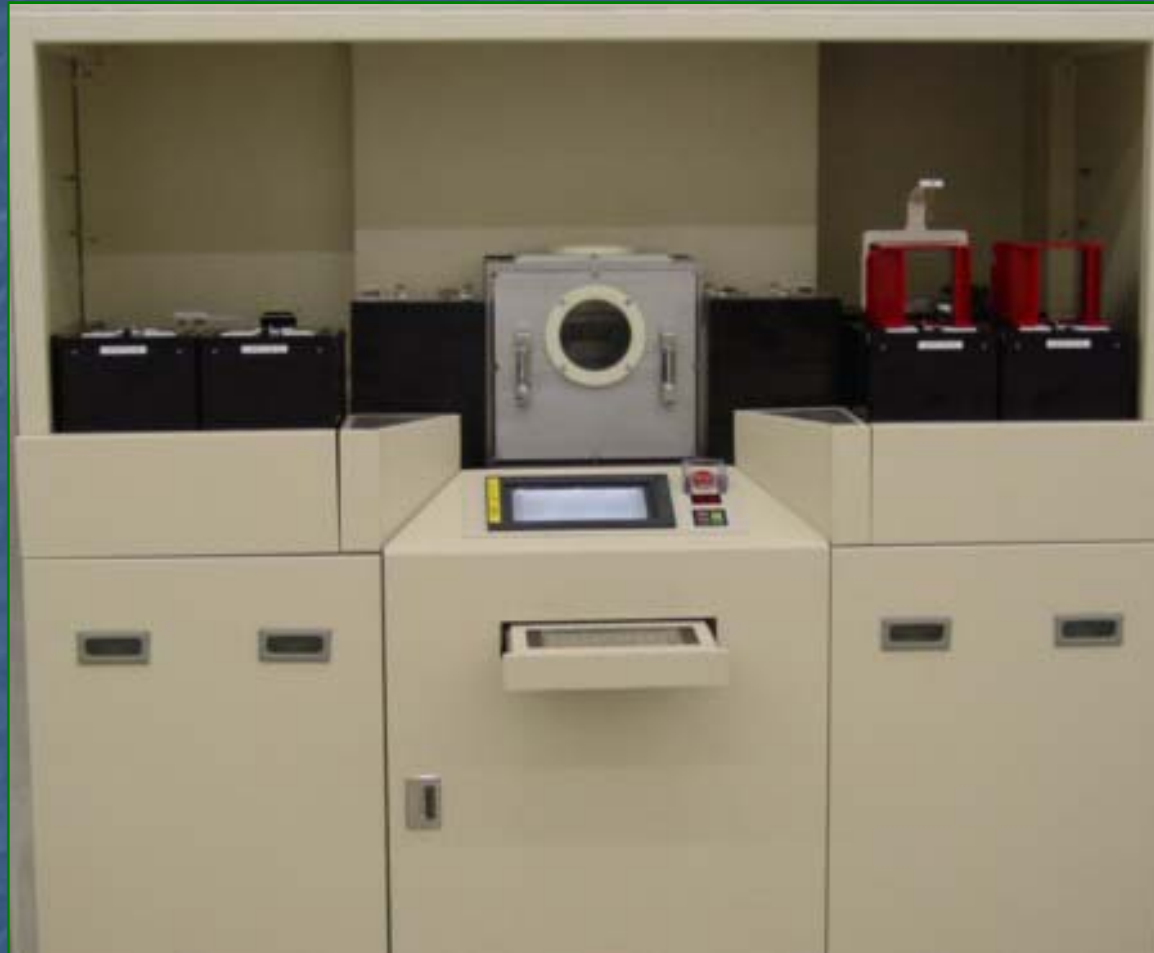
Medium current ion implanter NH-20SR
