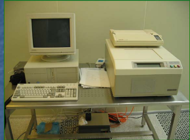
Omnimap RS-30 Four-point probe
