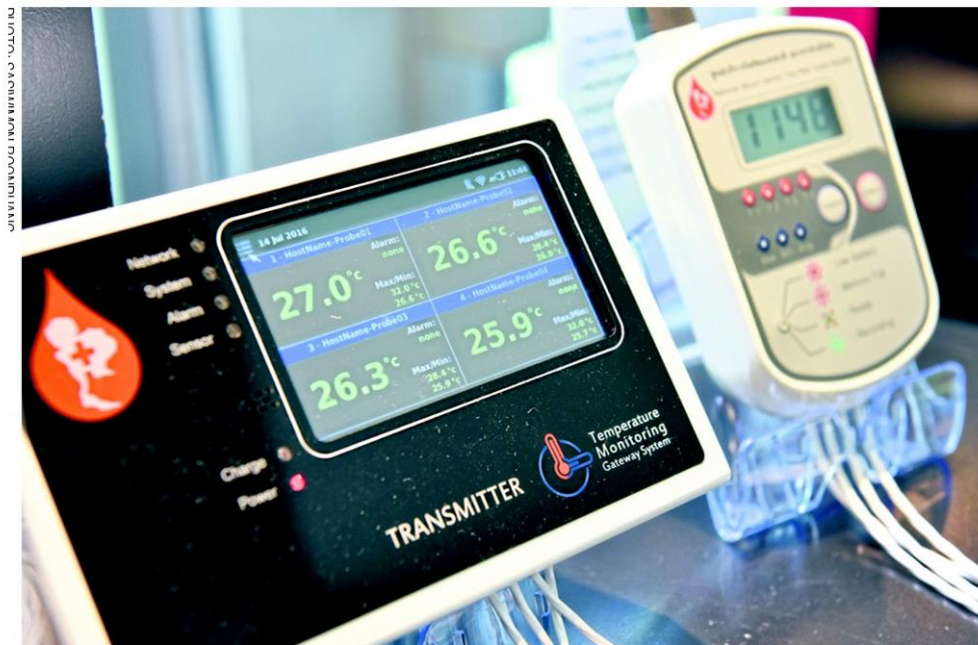
Mobile temperature data logger system has been used at Siriraj Hospital to ensure that blood and vaccine are kept at an appropriate temperature.
