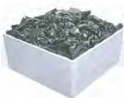
Crucible Filled with Solar Grade Silicon Feed Stock
