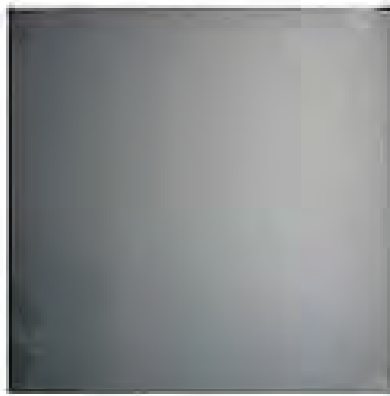
Mono Area with Small Amount of Multicrystalline Area
