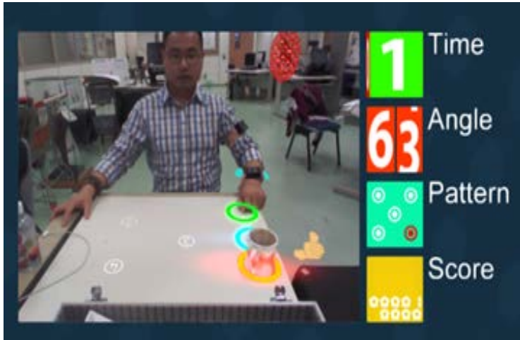
Upper limb tracking with MS Kinect + accelerometers with augmented reality game interface
