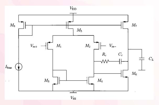
• Differential-pair input stage, frequency-compensation network, output-stage driver.
