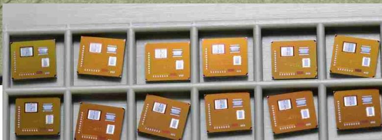
3-axis CMOS MEMS accelerometer
