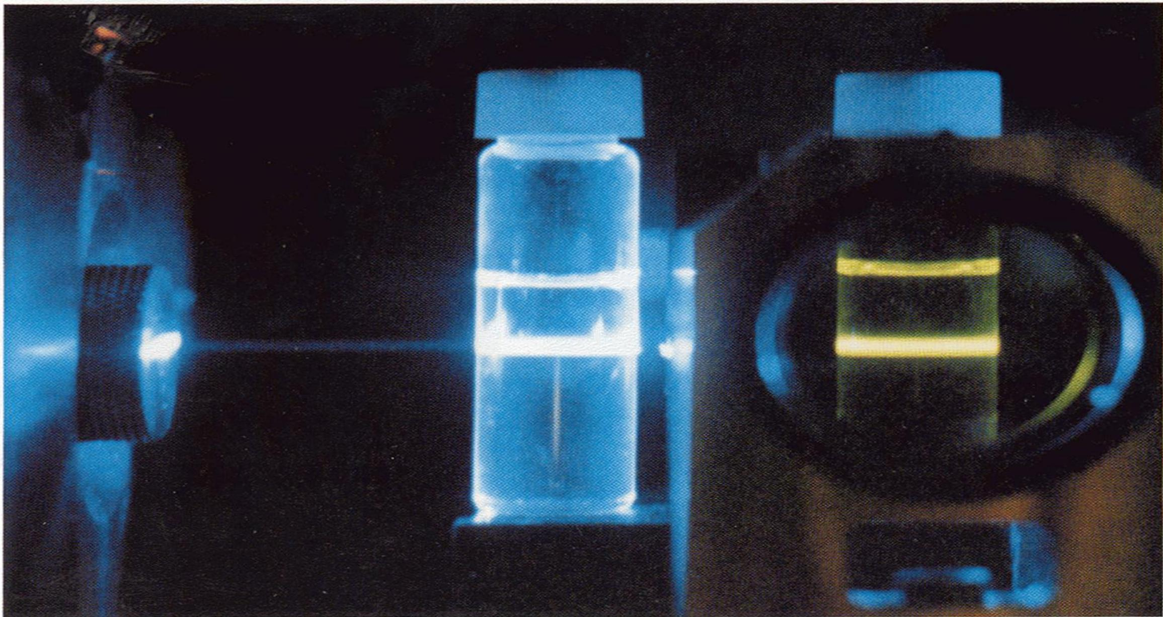
Raman scattering visible to the unaided eye, from a 488 nm laser beam passing through liquid cyclohexane. Left vial exhibits mostly Rayleigh scattering which obscures much weaker Raman scattering. Right vial is viewed through a 488 nm band rejection filter, which permits observation of longer wavelength Raman scattering.
