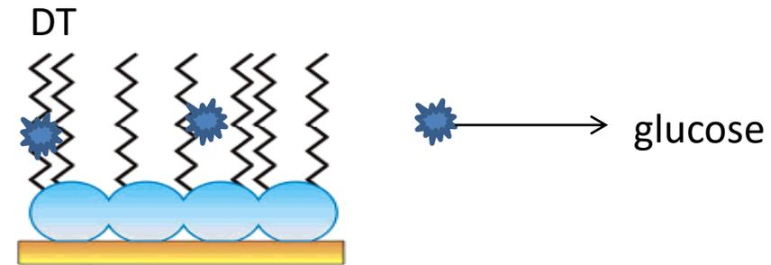
We have used a linker molecule 2 Thienyl Boric Acid that attaches to silver surface on one side as well as to D-Glucose on the other side
