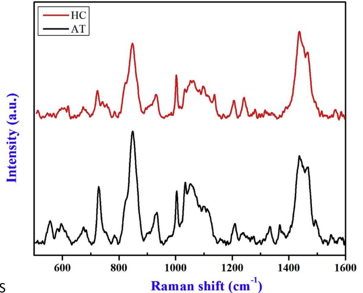
SERS spectra of active TB (AT) and healthy control (HC) samples with laser excitation wavelength of 785 nm
