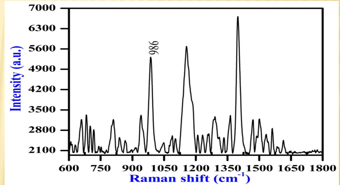
**SERS spectrum of 0.1M 2TBA+ 100µM D-glucose**
