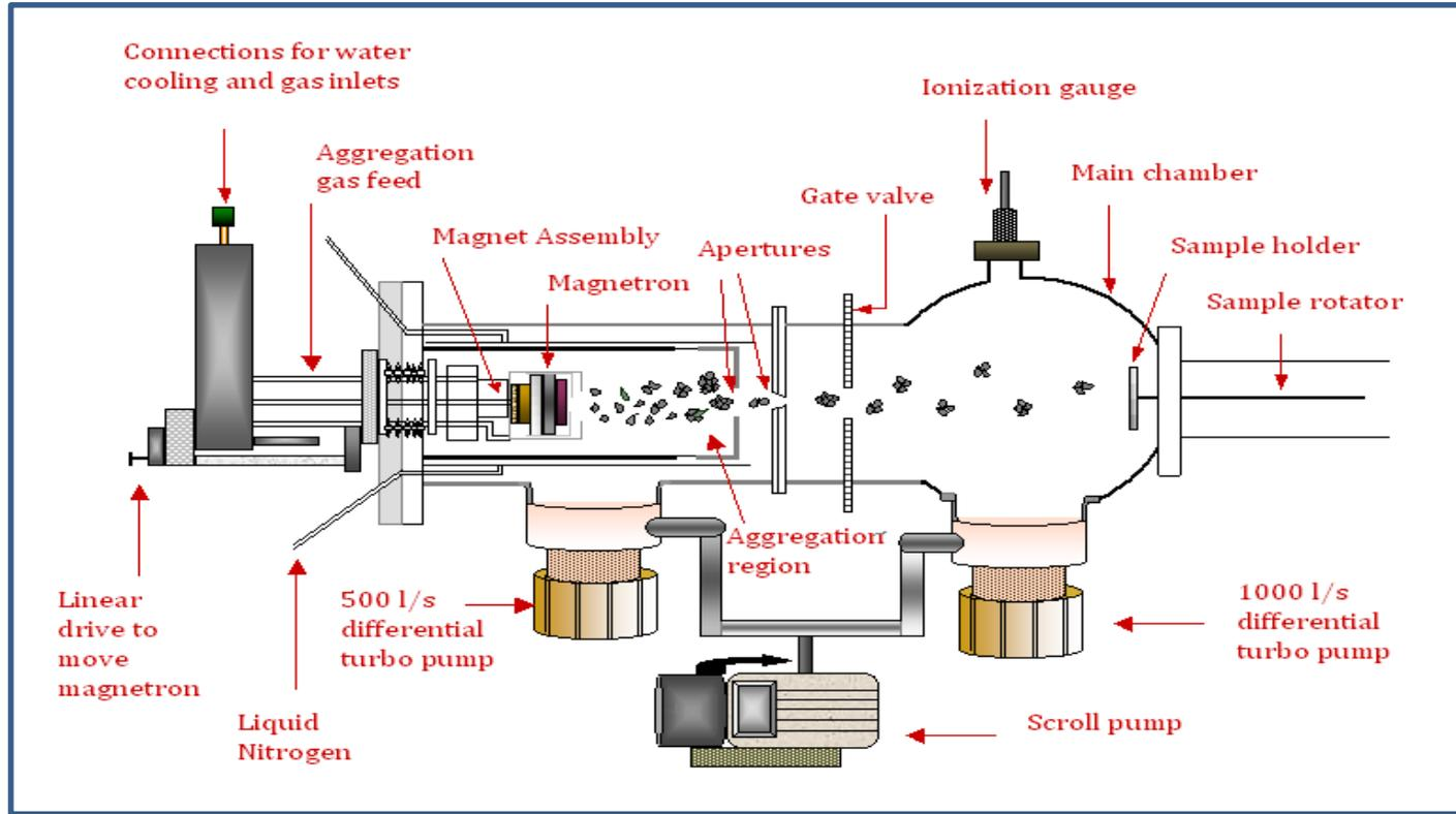
Block diagram of Nanocluster deposition system
