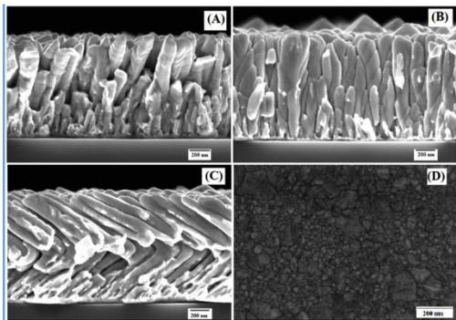
Slant, vertical zigzag nanorods and nano particles of Ag as SERS substrates
