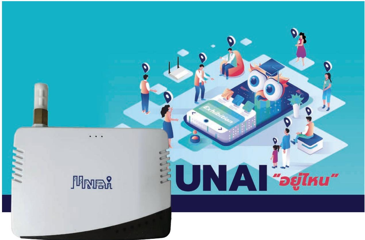
The signal receiving device or Anchor is a part of Indoor Localization System (UNAI Platform) developed to work with the transmitting device known as Tag to send signals to the computer server for identifying the tag's location and displaying the position and a route to the targeted objects for users.
