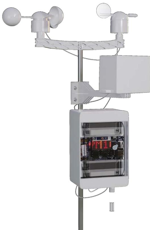
The weather station prototype was developed as an educational tool for the secondary school students to learn about new technology under the Data Science@School project. Learners are able to create a set of commands to control the operations of devices using Block-structured Programming just by dragging and dropping blocks through the KidBright IDE program on the KidBright board.
