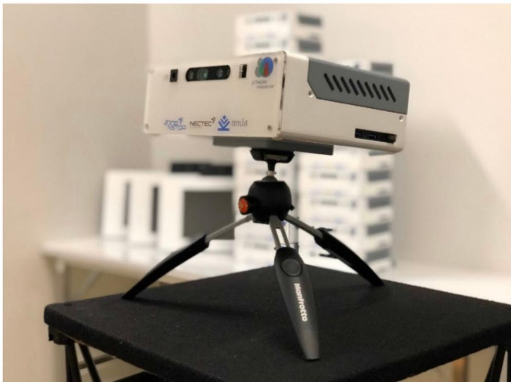
μTherm-FaceSense was developed to simultaneously measure multiple people's body temperature with no contact for just 0.1 seconds. Featuring a maximum screening range of 1.5 meters, the system uses infrared cameras combined with the automatic face detection technology to measure the temperature of people even covered by masks to prepare a preliminary screen for the COVID-19 infection.
